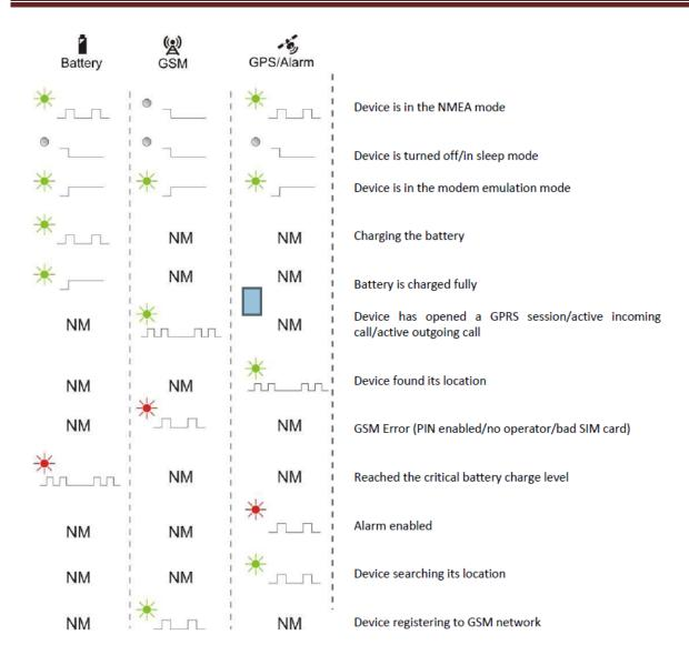
NM - means that it's no matter what LED indicator is blinking at the current moment.
